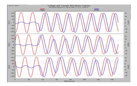
Waveform capture is also useful during steady-state conditions. The current wave shapes can show harmonic currents from nonlinear loads, and the voltage wave shapes show the distortion due to harmonic currents and transformer loading. It takes a large amount of memory to store raw waveforms. The memory size of a single 3-cycle waveform capture record is larger than the size of four hours of interval graph data (at one-minute intervals).
