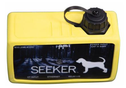
It is important to connect channel 1 voltage lead last since this will start the power-on process. This connection sequence will assure that all measured voltages and currents begin recording simultaneously and will prevent false event triggering that could occur during voltage lead or CT connection. The Status LED In the center of the Seeker will begin to display a color an pattern sequence.
