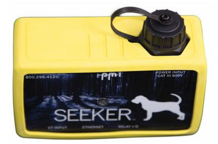
It is important to connect channel 1 voltage lead last since this will start the power-on process. This connection sequence will assure that all measured voltages and currents begin recording simultaneously and will prevent false event triggering that could occur during voltage lead or CT connection. The Status LED In the center of the Seeker will begin to display a color an pattern sequence.
