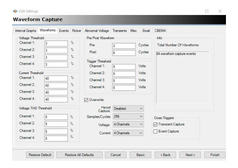
The default setting for triggering a current waveform is 40%. If you wish to capture more or less current waveforms, simply set this value higher or lower. If you do not wish to capture any waveforms based on variations in current, simply set this percentage to a very high level, so that it is unlikely that a waveform will ever be triggered by a current variation (the highest allowed trigger threshold is 900%).
