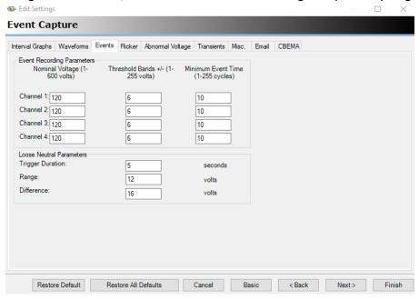
The minimum event time is not as critical. Ideally, this is set to a value larger than the slowest anticipated sag time. For example, if no sags (such as from motor starts, etc.) will take longer than 6 cycles for the voltage to drop to the sag value, the best minimum event time is 7 cycles. This will prevent multiple event changes from the same voltage sag. Otherwise, as the voltage drops lower and lower, past voltage trip points, events will continue to be triggered.
