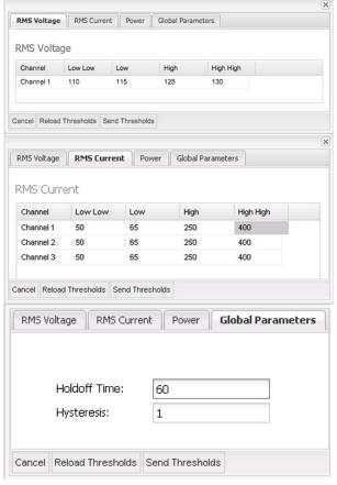
The Settings Configuration panel allows users to set thresholds for each channel and measure supported by connected devices. When used in conjunction with e-mail alerts, automatic e-mail notifications can be sent when trigger thresholds are exceeded.
